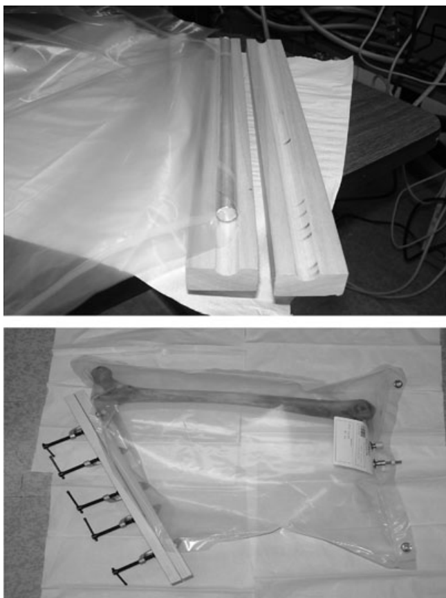
FIG. 2—Tedlar ® bag sealing device for bone vapor sampling.
