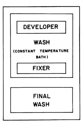
FIGURE 40.—The processing sequence in the preparation of X-ray films. The first solution is developer, which darkens the silver halide crystals in the exposed portions of the film emulsion. The developed film is washed for about two minutes before immersion in the fixer solution, which removes the unexposed silver halide crystals. A final wash removes all the processing solutions.
