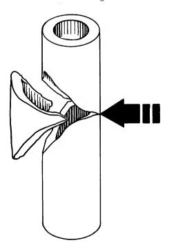
$F_{IGURE}$  49.—Schematic representation of bending fracture and the triangular fragment that may occur in such fractures.
