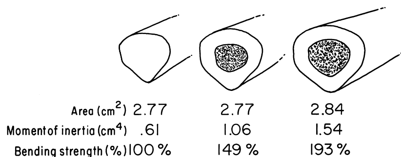
Figure 13 Moment of inertia properties of bone. Although the cross-sectional areas of bone in each of these three bones are roughly equivalent, their bending strengths are very different due to the differences in moments of inertia. This occurs as a result of the way bone is distributed in relation to the central axis of bending or rotation. The solid bone on the left has the same amount of bone (area) as the one in the center, but the latter has a higher moment of inertia because the bone is farther away from the central axis. Thus its bending strength is 50% greater. Similarly, the bone on the right has only slightly more bone area than the one in the center, but its moment of inertia is again 50% higher, making it 30% stronger under bending stress. Reprinted with permission from Einhorn, T. A., Ariza, M., and Goldstein, S. A. (1992). "Bone-Fragility: The Biomechanics of Normal and Pathologic Bone." Sandoza Pharma Ltd. Monograph.
